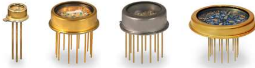
Figure 2. Some kinds of APD's as used in particle and nuclear physics. The device at far left is the APD used in our study.
